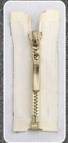
901A-176 No.5(or No.3) Aluminum zipper, mirror-polish teeth, golden color, 0/E, A/L, 901D-451 slider normal
