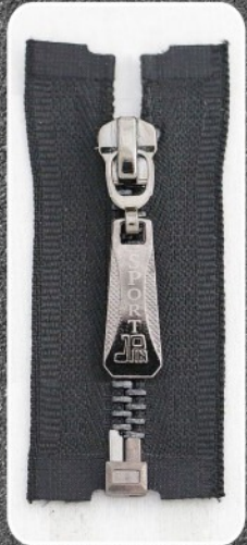
901A-171 No.5 Aluminum zipper, black nickel teeth, 0/E, A/L, with laser slider
