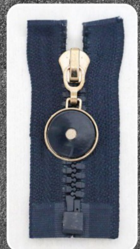
901A-157 No. 8 plastic zipper, Two-layer teeth, O/E, A with plastic Pin&Box
