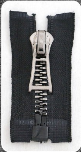
901A-128 No. 5 (or No. 8) plastic zipper, Imitation metal teeth black-nickel color, O/E, A/L, with plastic Pin&Box
